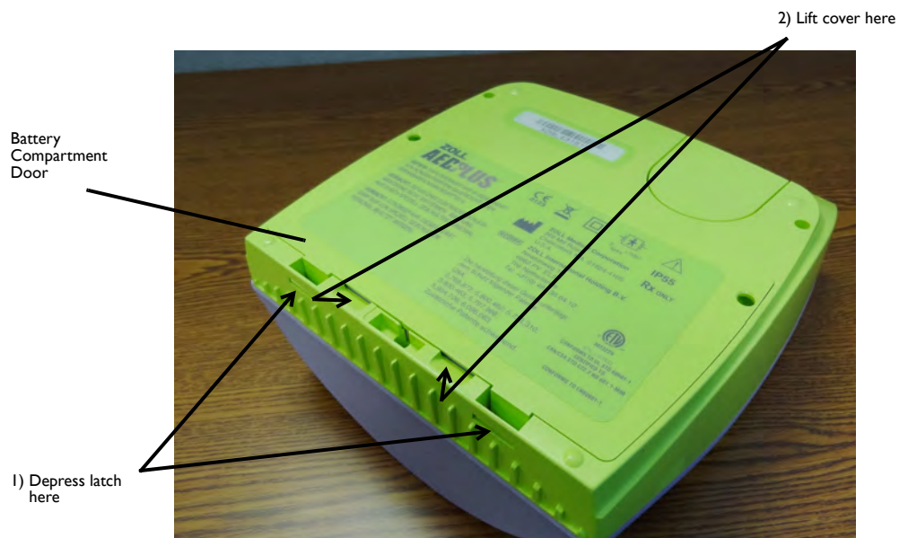
Figure 7: Removing the Battery Compartment Door
